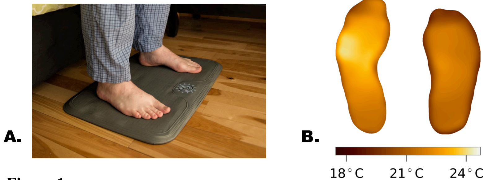
Figure 1. Approximately 25,000 thermograms were collected as part of the trial. A. Wireless foot mat with thermometric coverage across the plantar surface B. B. High-resolution thermograms collected with each use.
