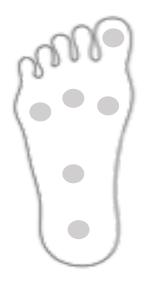
The temperature data collected by the mat are automatically analyzed for temperature differences, or asymmetry, between the left and right feet at six locations consistent with the approach most common in the literature [5-7].
