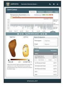
The thermometric data collected by the mat are referred to as scans and are securely transmitted and accessed.
